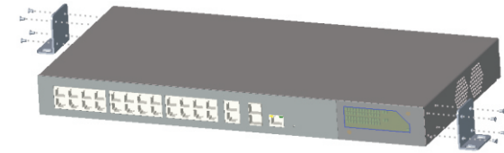
Figure 2-3 Hangers installation diagram
