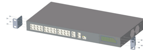
Figure 2-1 Install hangers diagram
